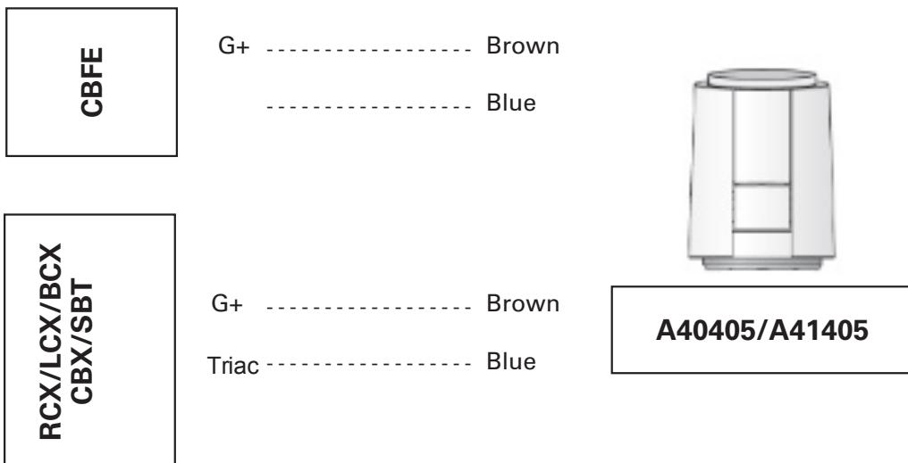
CBFE = Fan coil control box [EC-motor]
