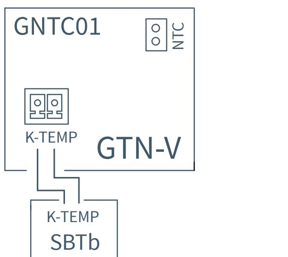
**SBTb** = Valve actuator control unit
